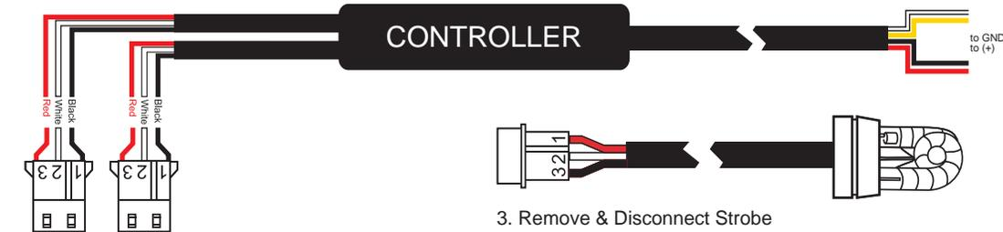
2. Connect LED Kit connectors to strobe extension cables.
