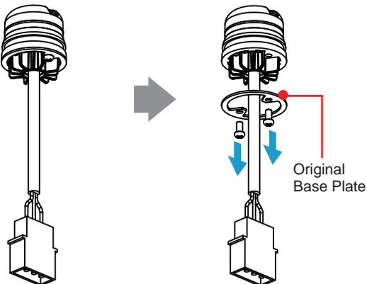
2. Secure Flange Plate to lighthouse base with screws.
