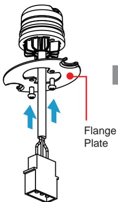
3. Use mounting flange to mark wire and screws holes to drill.
