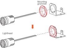
2 Ensure that the optical stripes are aligned vertically.
