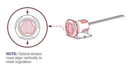
Secure the BRACKET onto the desired mounting surface with screws.
