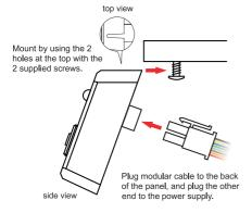
NOTE: Connect only the RED and BLACK wires to the power supply wiring harness.
